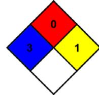
NFPA fire hazard : 0 - Materials that will not burn under typical dire conditions, including intrinsically noncombustible materials such as concrete, stone, and sand.
